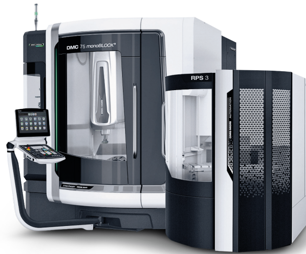
DMG MORI DMC-75 palletised monoblock (3 pallet)
